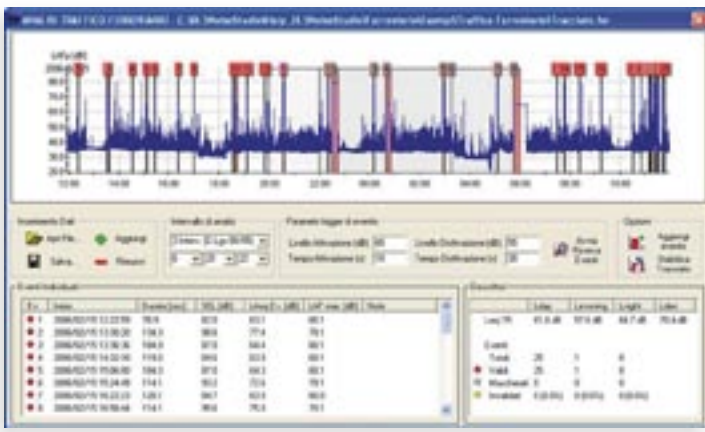
DL5 Noise Studio: Railway traffic module: 24-hour analysis with automatic transit search.
